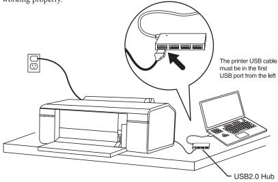
**Note:** The printer and Autoloader must both be connected to your PC using the included hub in order for the Autoloader software to work properly.
